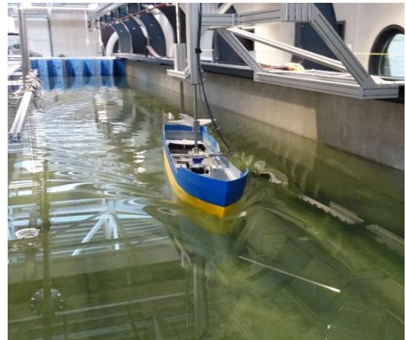
Figure 64. Model of JUREN-AE in towing-tank at Maritime Testing Facilities in Leer.
