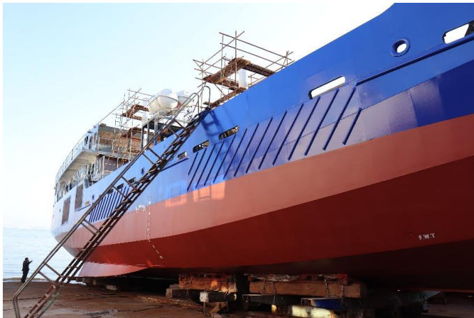
Figure 67. Delta-shaped keel at starboard side, Korea 2024.
