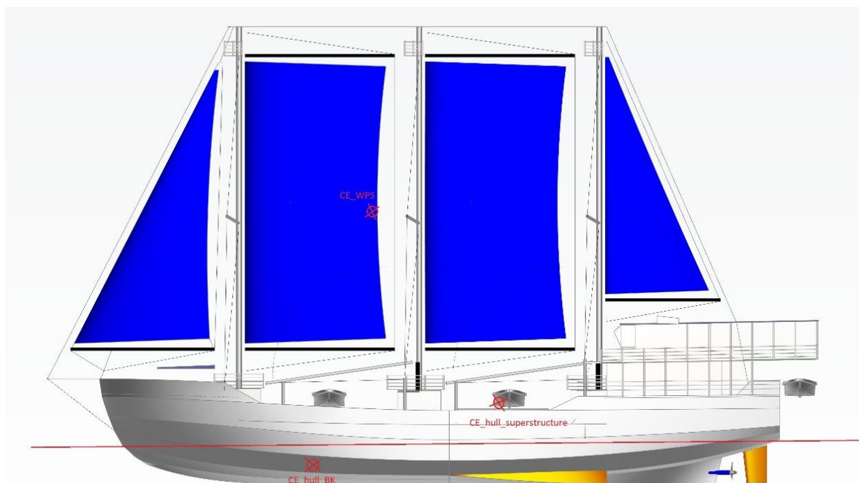
Figure 50. parametric 3D-Model used for initial design and calculations created within CAESSES.
