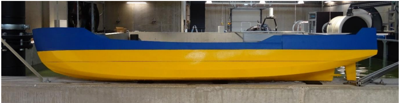
Figure 51. Towing-tank model with center-skeg and rudder, side-view.
