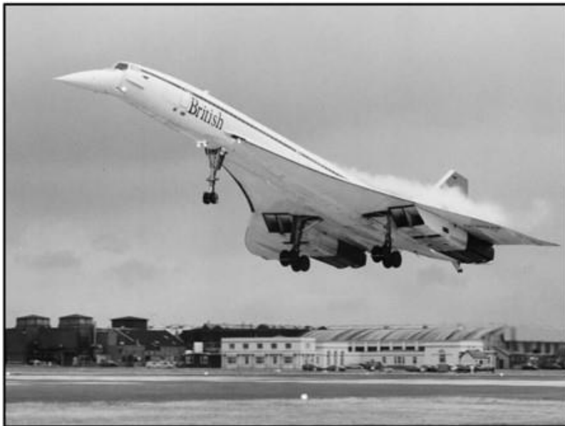
Figure 3. Vortices forming above the wings of Concorde during landing and take-off.
