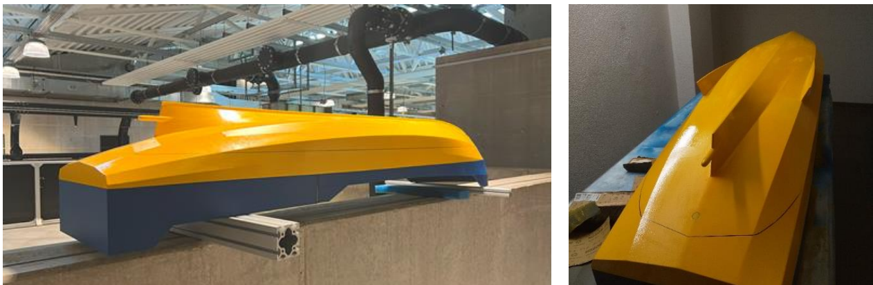
Figure 52. RMI-Design – towing-tank model with bar keel (left) and delta-shaped bilge-keels (right).
